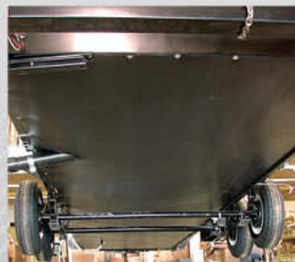
The Heated and Enclosed Underbelly
