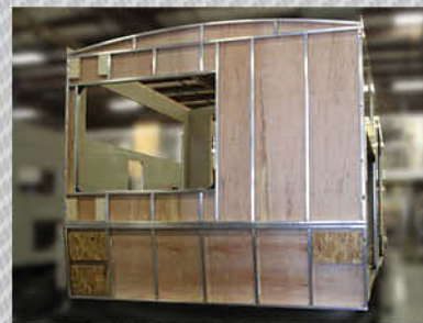
Double welded aluminum cage construction in walls, roof and floors.
